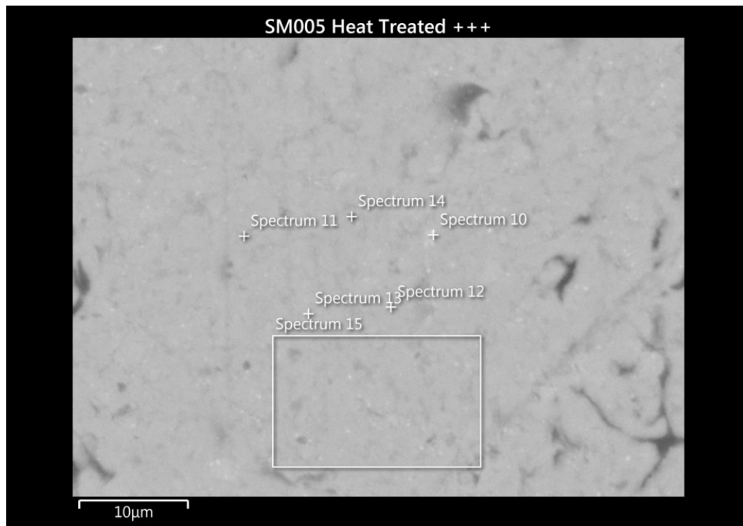
Figure 7: Much higher magnification (5000X) of the heat-treated aluminum alloy sample.
